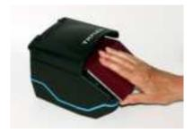
The reader was designed to hold a document in a natural semi-opened position. This hands-free function allows you to release the document and focus on the traveler.
