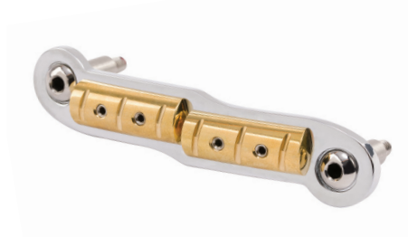
RSD J-BRIDGE Two movable brass saddles bolted to a cold rolled steel base provides an articulate tone with more punch, attack and continuity than its predecessor. The J-Bridge lets the sound of the guitar ring through and gives a stronger primary note.
