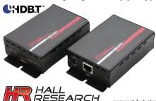
The UH-1BTX extends any HDMI or single link DVI video signal up to 330 ft (100 m) over inexpensive Cat5e or Cat6 cable using HDBaseT technology. This is currently the longest distance achievable for digital video over twisted pair. Video and embedded audio signals are transmitted without any compression to the remote for a 100% identical reproduction. The UH-1BTX consists of a kit of
