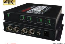
The Fiberlink 3514 series supports 4 channels of independent 3G/HD/ SD-SDI or DVB-ASI, with or without embedded audio and data, and transmits it over one single mode or multimode fiber. When using all four inputs, Fiberlink 3514 supports 4K/UHD resolutions at 60 fps. Fiberlink 3514 is capable of transmitting two 4K/UHD signals at 30 fps simultaneously. Each receiver features four reclocked, non-inverting BNC outputs. The 3514 Series is compli-
