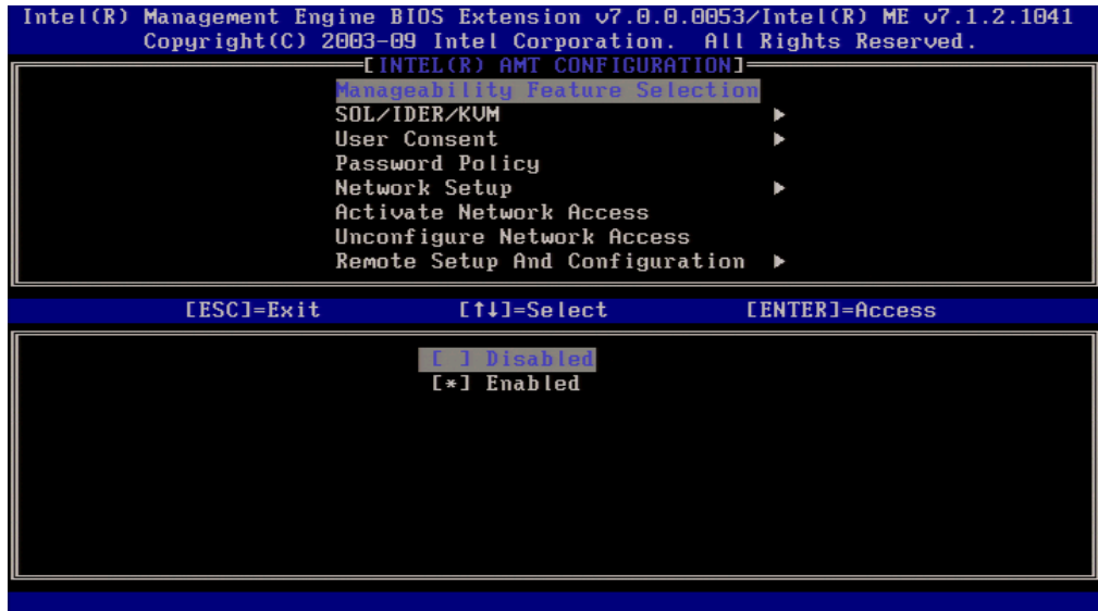
Figure 9. Intel AMT Manageability Feature Selection Screen
