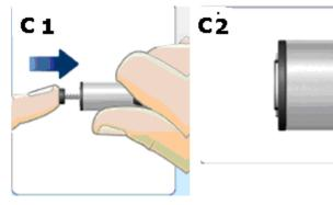
C. Push in the piston rod, by gently pressing the piston rod head (see Figure C1) in until it stops and looks like Figure C2.
