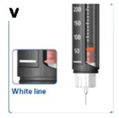
V. Do not try to inject an insulin suspension (white and cloudy insulin) if the rubber stopper (plunger) is below the white line on the holder as in Figure V. The glass ball inside the PenFill cartridge must have enough space to mix the insulin.
