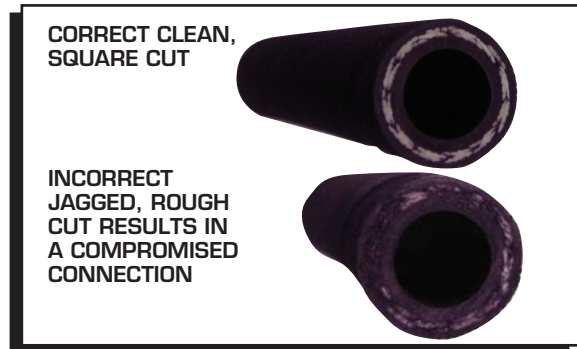
Figure 5 Severing the Hose Properly.
