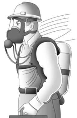
Self-Contained Breathing Apparatus (SCBA) Atmosphere-supplying, or Supplied-air respirator (SAR), which provides clean air from an uncontaminated source Needs to be fit tested APF=10,000
