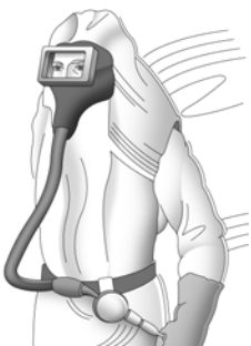
Abrasive Blasting Respirator; Atmosphere-supplying respirator Full Facepiece Elastomeric APF=25/1,000* Needs to be fit tested; Continuous flow
