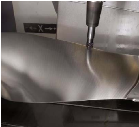
Turbine blade during machining. Face milling on the other side with rotation around the X axis.
