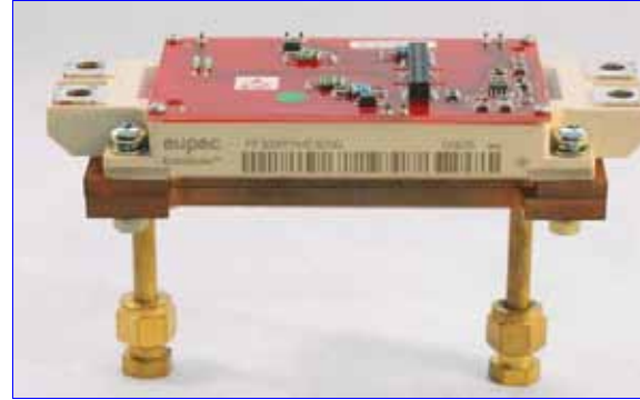
Figure 3: VDF-cooled copper convoluted fin cold plate (Case E1, E2).
