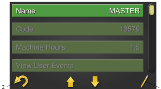
Illustration 14: Editing an Operator's Information (1) Enter the Editing Screens (2) Return to the Previous Menu
