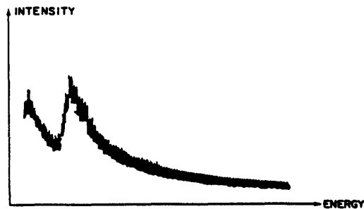
Fig. 4. Electron transmission spectrum of carbon directly detected by photodiode array.
