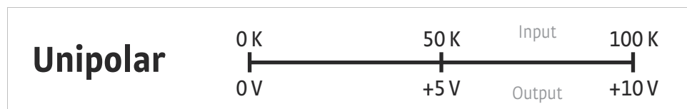
FIGURE 5-4 Output with polarity parameter set to unipolar
