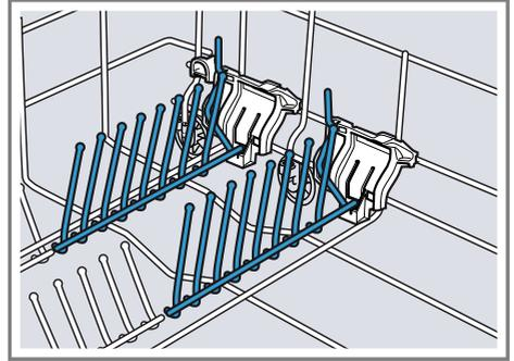
For easier storage of pans, dishes and glasses, you can fold the folding plate supports.<sup>1</sup>
