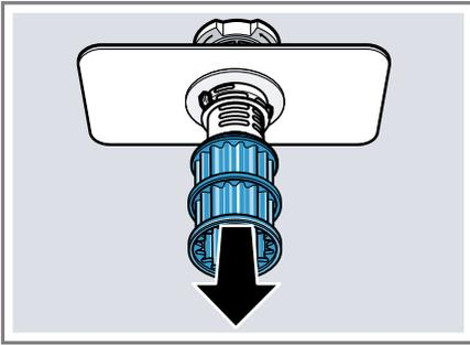
4. Press the locking pieces together and remove the coarse sieve remove upwards .
