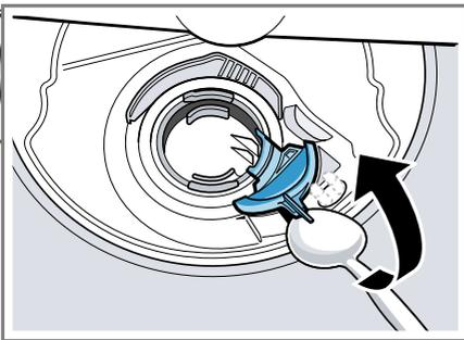
6. Lift the pump cover diagonally inwards and remove it.
