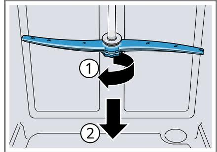
2. Pull the lower spray arm upwards.
