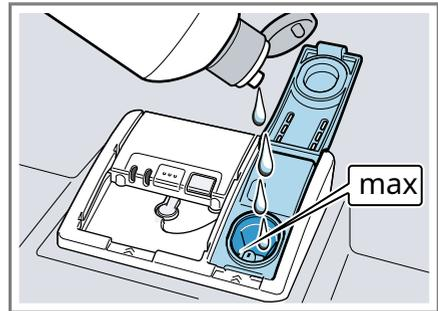
3. If rinse aid has spilled over, it must be removed from the rinse aid container.
