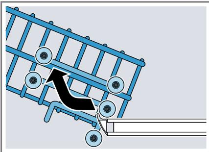
3. Place the basket on the upper rollers (position 3) or the lower rollers (position 1).
