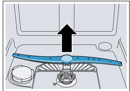
3. Check the nozzles of the spray arms for blockages under running water and remove any foreign objects.
