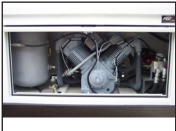
H150 air compressor with PTO/hydraulic drive. 127 CFM with a 23 or 38 gal. tank.
