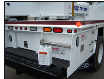
Optional rear step and grab handle for easy access to the bed.
