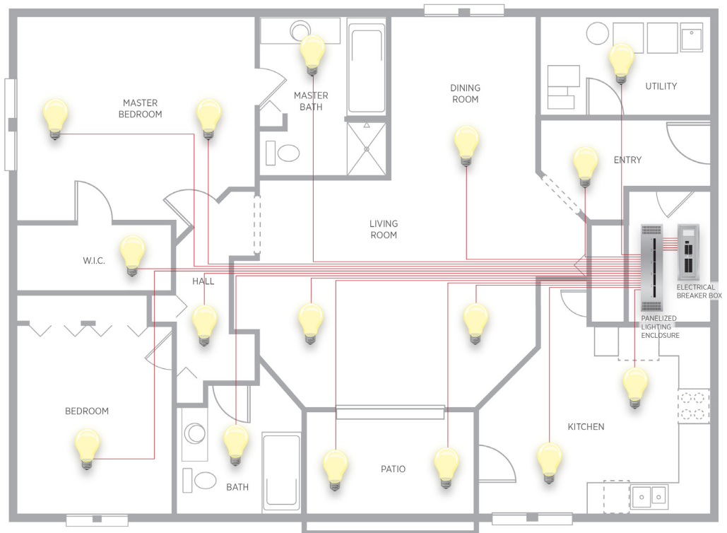
Figure 3. Centralized Panel Design Example
