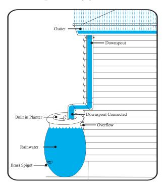
The Castilla Rain Barrel system is an easy way to collect and store natural rainwater.
