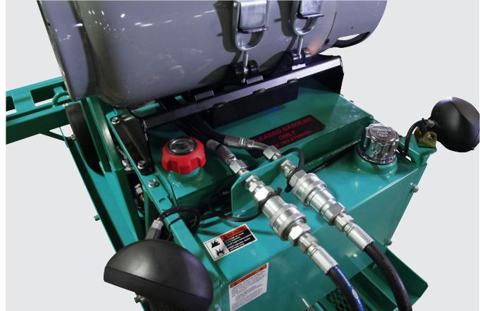
**Quick connect couplers** provide fast teardown and assembly. Allows easy storage of power unit.
