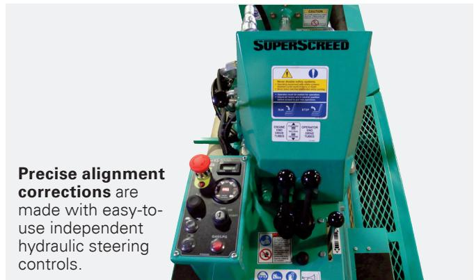
**Precise alignment corrections** are made with easy-to-use independent hydraulic steering controls.
