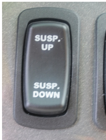
Figure 7-5: Main Suspension Switch
