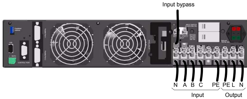
Figure 2-21 Cable connection for 3-input 1-output, split-bypass configuration
