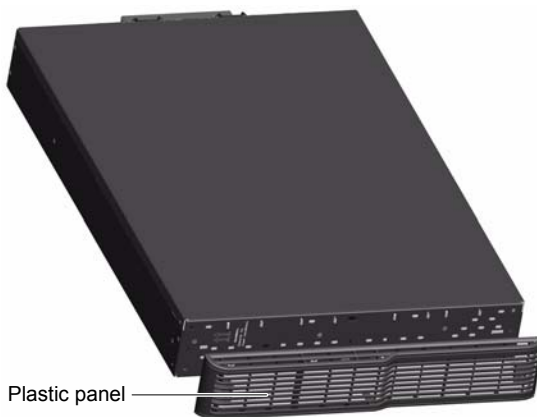
Figure 8-2 Removing the plastic panel
