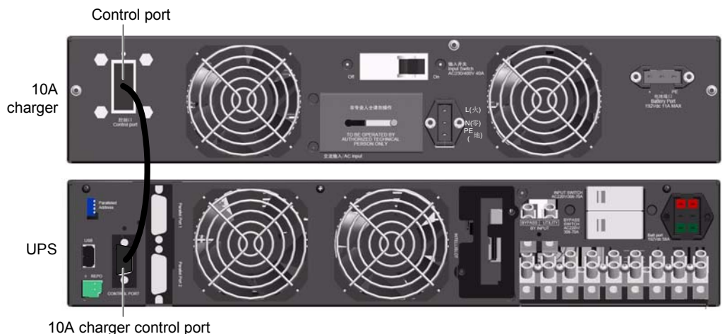
Figure 2-28 Cable connection of 10A charger
