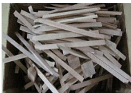
Some timber offcuts previously disposed of as waste are instead reused as angle rafters (reinforcing materials inside guitar bodies)
