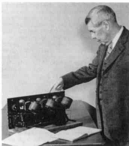
Figure 1. Professor L.A. Hazeltine and the prototype neutrodyne receiver, which was presented to the Smithsonian Institute in 1956.
