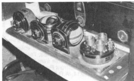
AK breadboard home brew with original AK parts.
