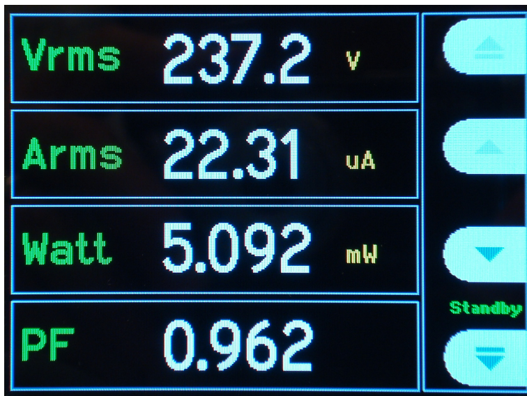
Figure 19: PA1000 measuring 5 mW in front-panel standby mode
