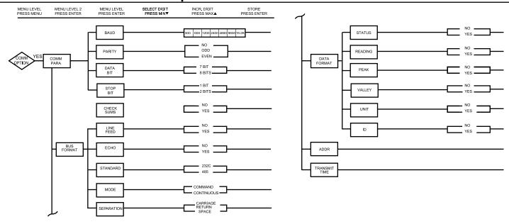
Figure 3.10 Flowchart for Communication Option
