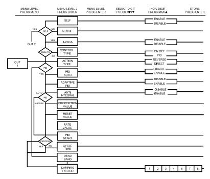
Figure 3.6 Flowchart for Output 1
