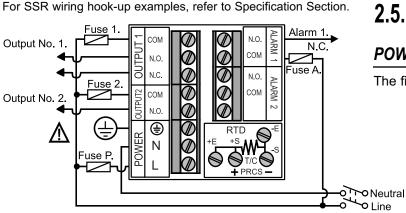
Figure 2.5.1 Power Wiring Hookup
