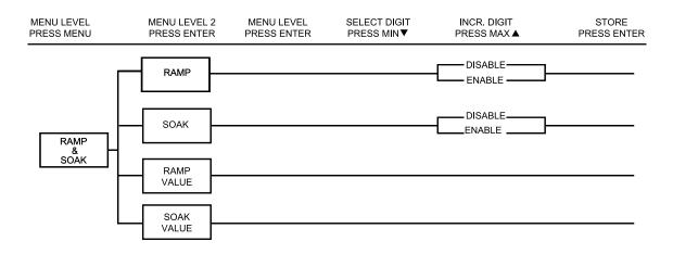
Figure 3.8 Flowchart for Ramp & Soak
