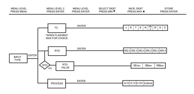
Figure 3.2 Flowchart for Input Type
