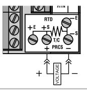
The figure shows the wiring hookup for Process Voltage 0 - .1 V, 0 - 1 V, or 0 -10 V. When configuring your controller, select Process type in the Input Type menu (see part 3).
