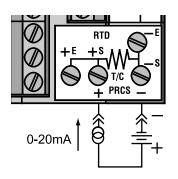
The figure shows the wiring hookup for Process Current 0 - 20 mA.
