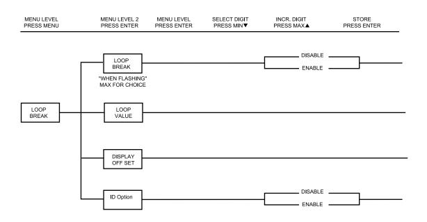
Figure 3.5 Flowchart for Loop Break
