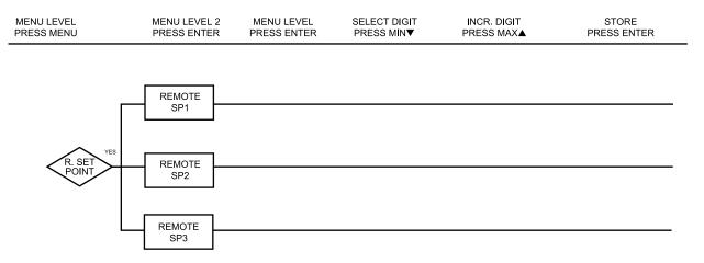
Figure 3.11 Flowchart for Remote Setpoint
