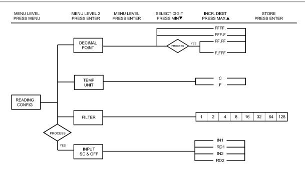
Figure 3.3 Flowchart for Reading Configuration
