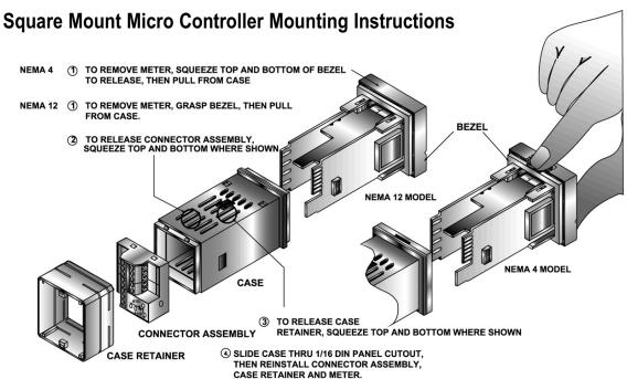
Figure 2.1a — Mounting the Square Mount Controller
