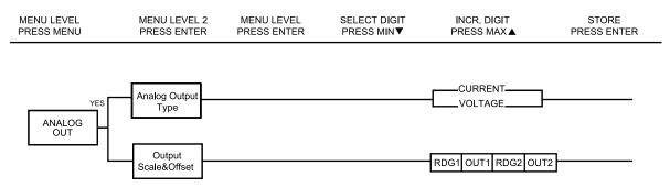
Figure 3.9 Flowchart for Analog Output Option
