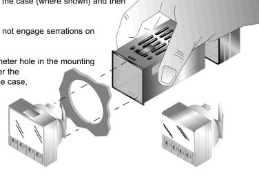
Figure 2.1b — Mounting the Round Mount Controller
