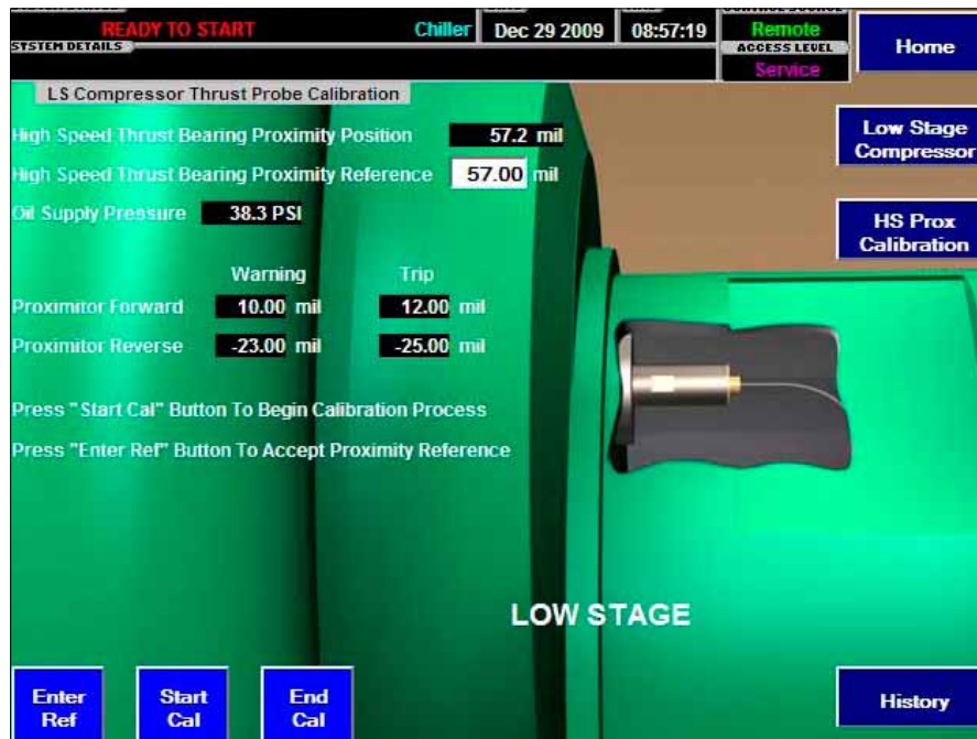
FIGURE 48 - HS PROXIMITY CALIBRATION SCREEN
