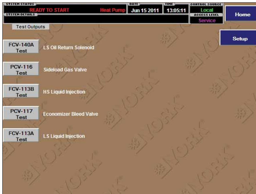
FIGURE 58 - TEST OUTPUTS SCREEN
