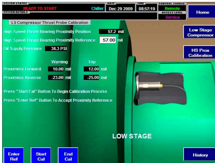
FIGURE 37 - LS PROXIMITOR CALIBRATION (LOW AND HIGH STAGES) SCREEN
