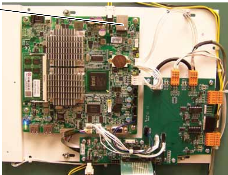
Bottom view of Quantum™ LX controller board
