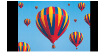
A 16:9 transmission , with a 4:3 picture in it. Dark bars are added at the sides of the transmission
