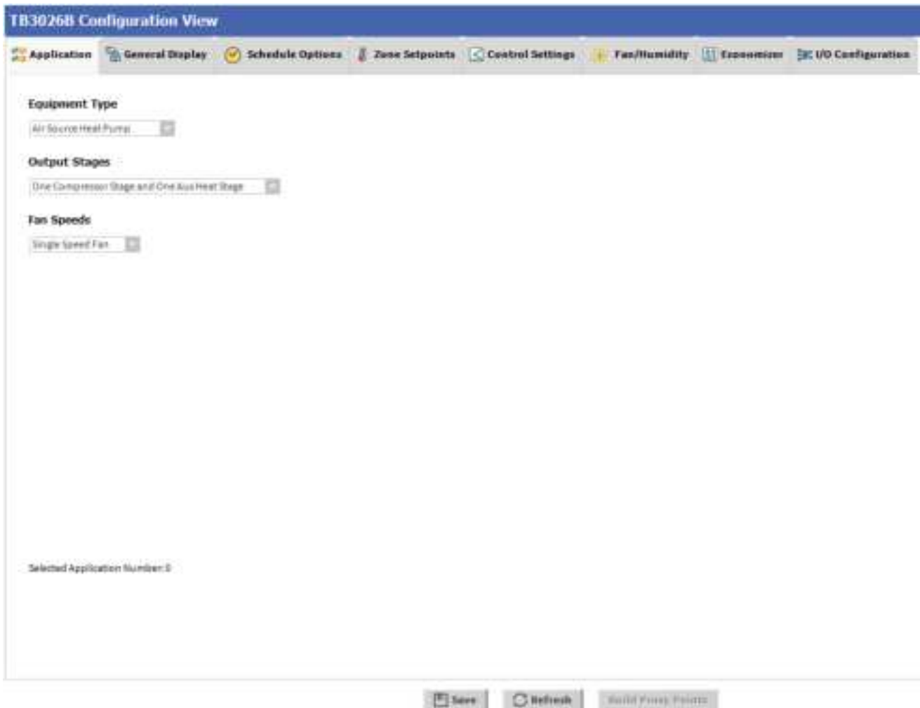
Figure 43: Air Source Heat Pump Window
