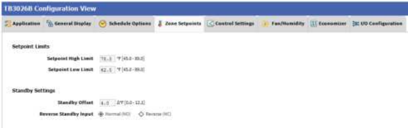
Figure 47: Zone Setpoint Screen (Setpoint Mode)
