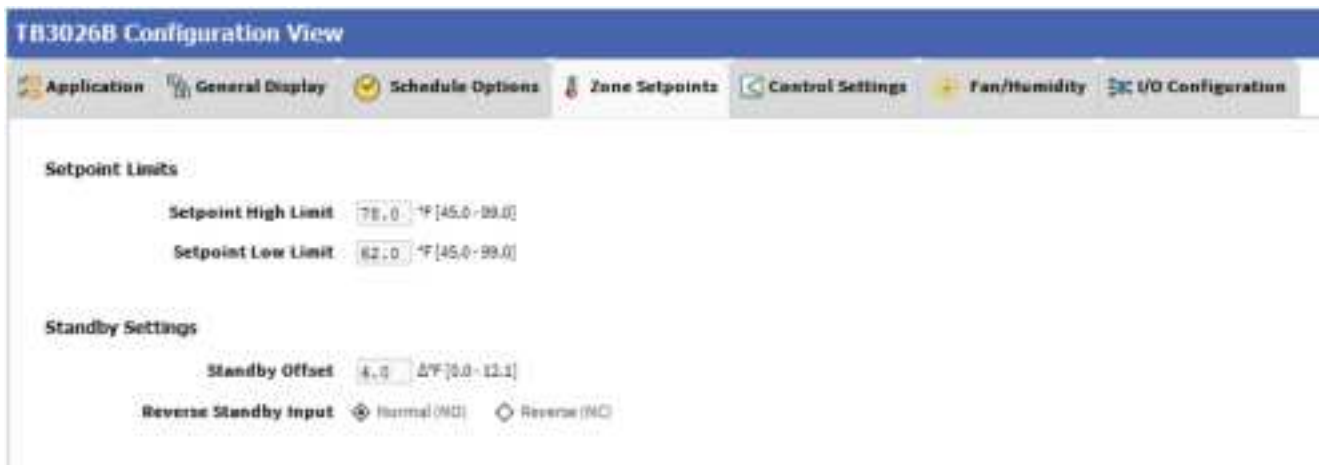
Figure 67: Zone Setpoint Screen (Setpoint Mode)
