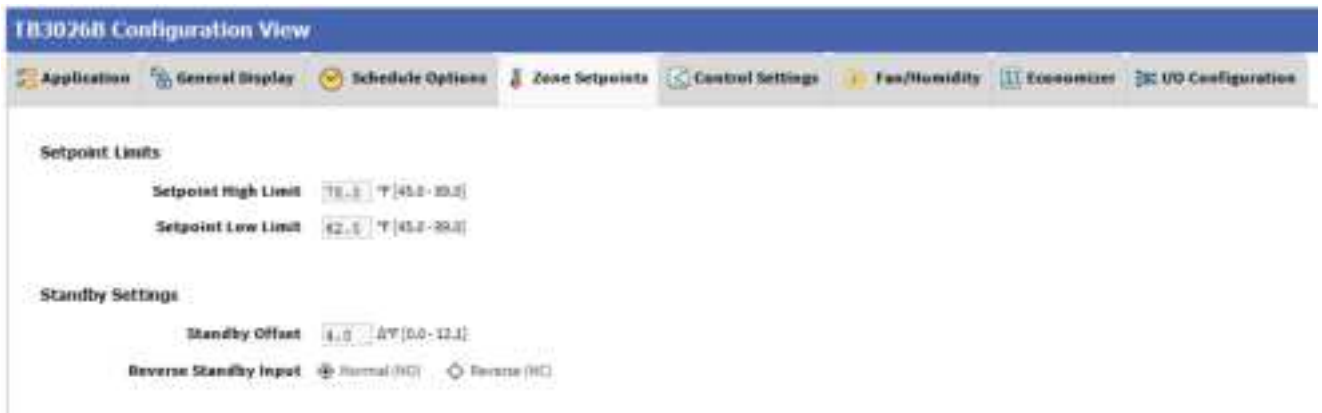
Figure 37: Zone Setpoint Screen (Setpoint Mode)
