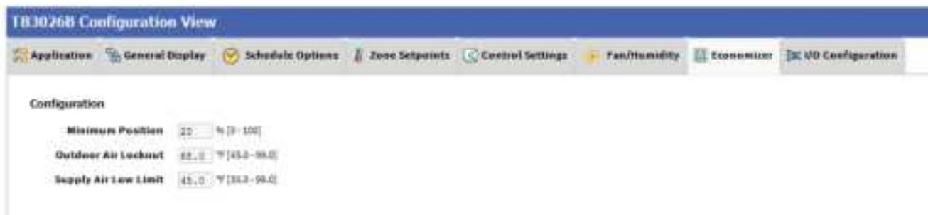
Figure 50: Economizer Screen (Air Source Heat Pump)
