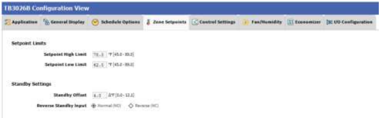
Figure 57: Zone Setpoint Screen (Setpoint Mode)
