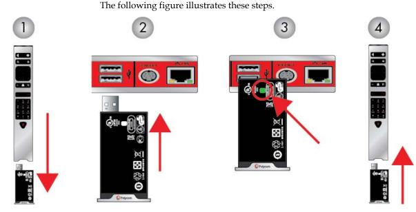
If you have a RealPresence Group 700 system, you can also recharge the battery using the USB port on the front of the system.
