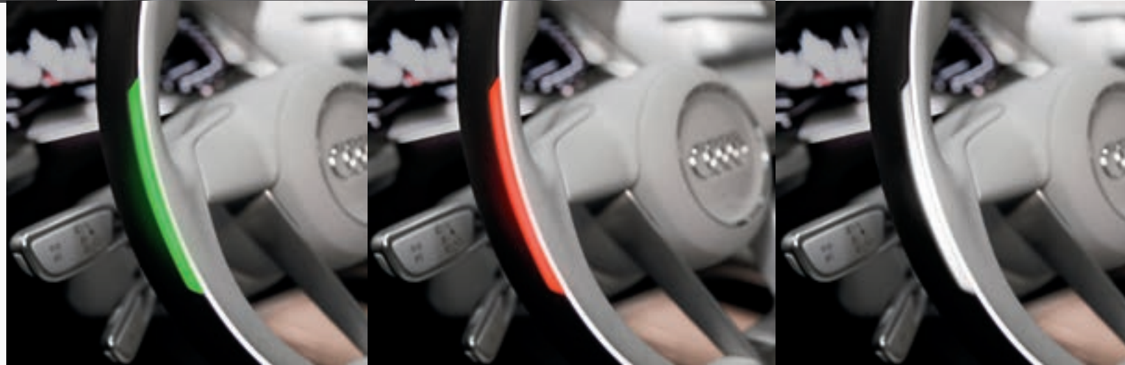
→ Green light along the steering wheel could signal to the driver: Piloted driving is active, the car is now steering autonomously.
