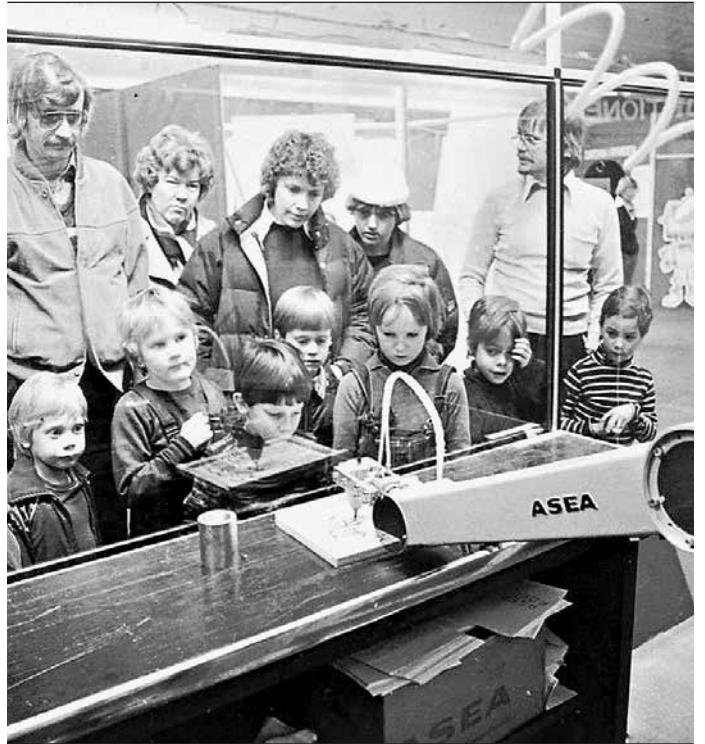
3 ASEA's IRB 6 was first presented in 1974. It had 5 axes and a payload of 6 kg. Many of the 1,900 examples built are still in use today.
