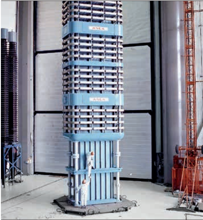
2 An early 1980s HVDC thyristor valve for the Inga – Shaba intertie project in Zaire (today, Democratic Republic of Congo).
