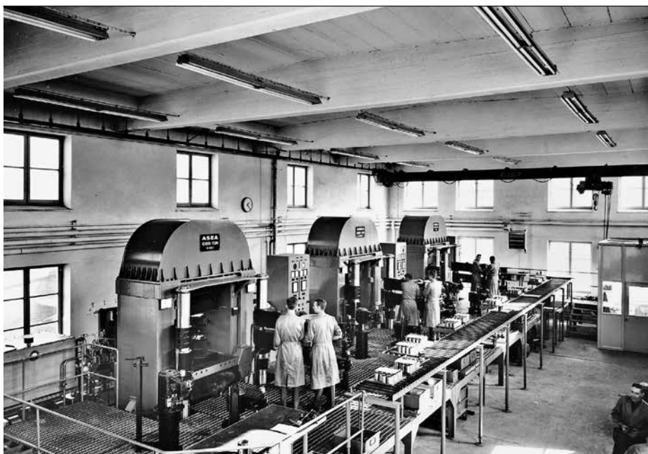
1a Starting in 1949, ASEA launched a top secret project for the creation of synthetic diamonds. The first success was achieved in 1953 when a pressure of 8.4 GPa was maintained for an hour and the first diamonds were obtained. The project was kept so secret that results were not reported until the 1980s.
