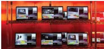
Temperature Test Extremely high or low temperatures tests ensure laptops' functions consistently for users everywhere.
