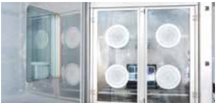
Altitude Test This tests the ability to survive extremes of altitude encountered in shipping by air or air travel.
