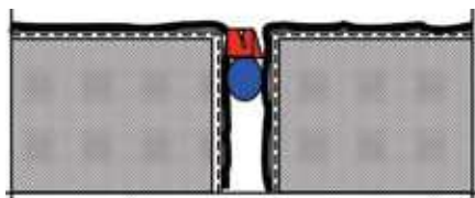
Fig. 1 Existing distressed sealant joint
