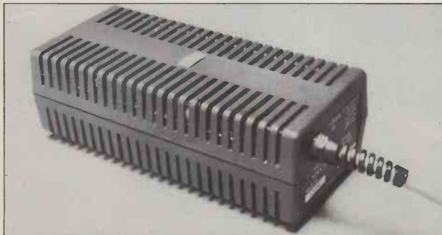
The main power supply is housed in its own well-ventilated casing.
