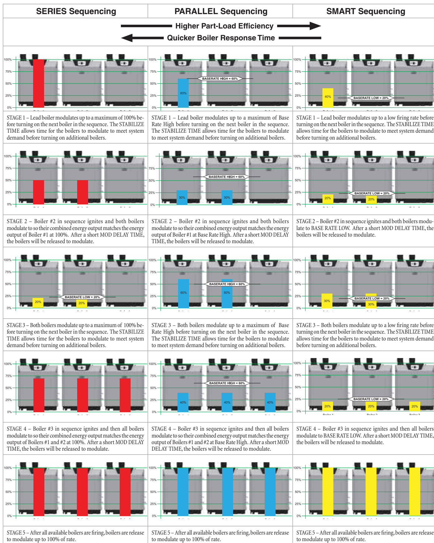
Figure 29 SlimFit sequencing options — SMART, PARALLEL or SERIES (examples shown for 3-boiler network)
