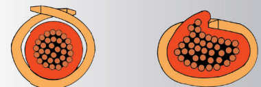
Insulation is not securely held
