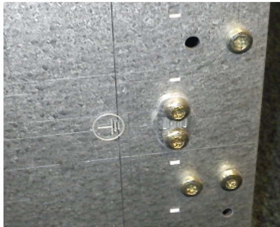
Figure 19: Earthing point 7U-chassis
