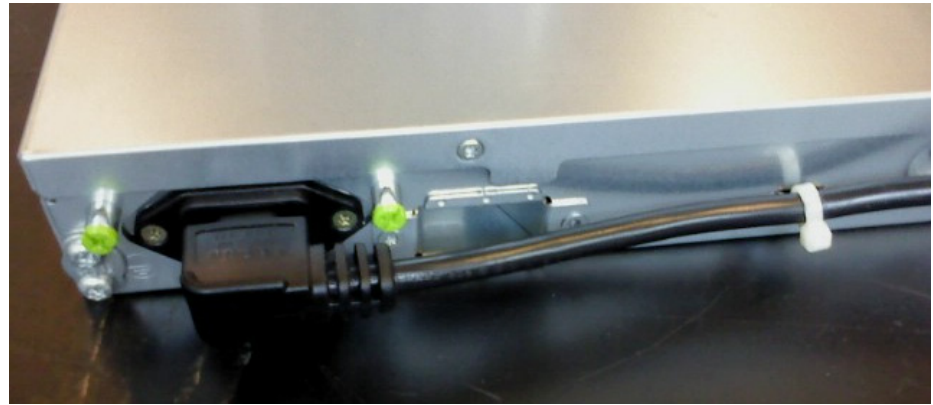
Figure 30: Secure Main cables
