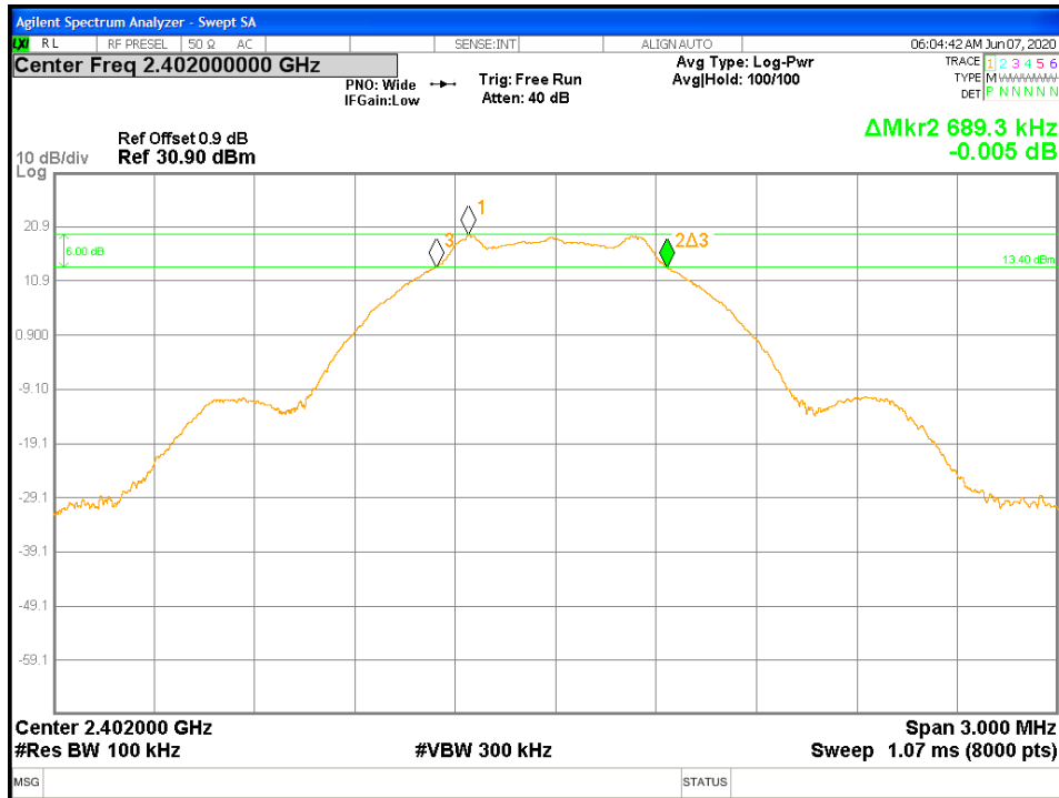
Figure 5: DTS Bandwidth-Transmitter -2402 MHz
