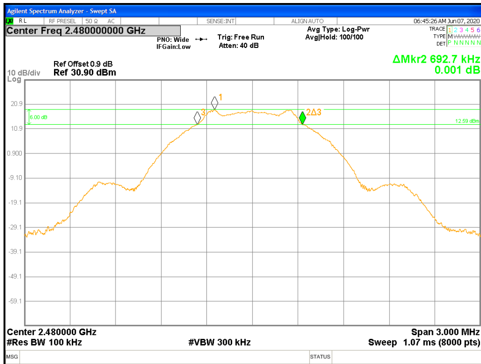
Figure 7: DTS Bandwidth-Transmitter -2480 MHz
