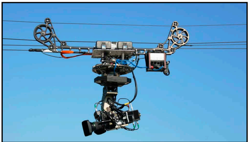
NBC Sports' "BATCAM" is a cable-supported, self-powered moving Panasonic AK-HC1500G HD box camera that goes from 0 to 60 mph in 1.5 seconds, reaching speeds in excess of 100 mph.
