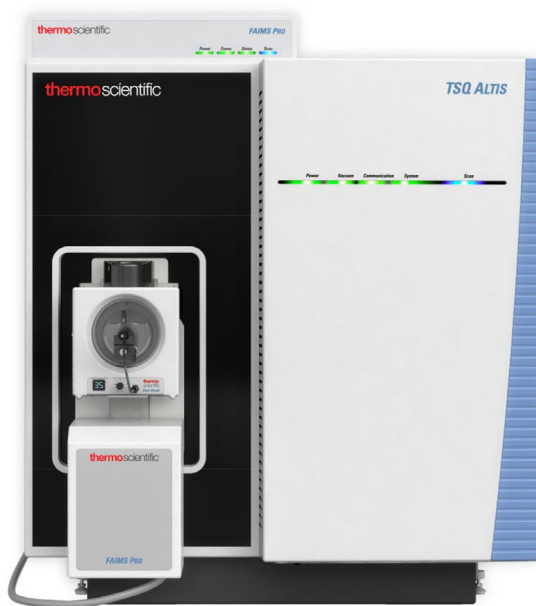
Figure 1. EASY-Spray ion source and FAIMS Pro interface mounted to TSQ Altis triple quadrupole mass spectrometer
