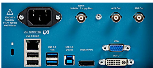
The I/O you need to connect the 6 Series MSO to the rest of your design environment.
