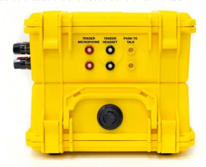
**TENDER HEADSET** - This is the dual banana jack (color-coded black) that functions as both an output (earphone) and input (microphone) for the tender as controlled by the PUSH-TO-TALK BUTTON and PUSH-TO-TALK JACK. Using this connection, the tender can be wired in either 2-Wire or Full Duplex (4-Wire) mode regardless of the mode used for the diver.
