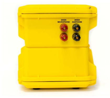
**DIVER MICROPHONE** - This is a dual 5-way binding post jack (color-coded red) that functions as both an output (earphone) and input (microphone) for the diver as controlled by the PUSH-TO-TALK BUTTON and PUSH-TO-TALK JACK. Using this connection, the diver can be wired in either 2-Wire or Full Duplex (4-Wire) mode regardless of the mode used for the diver.
