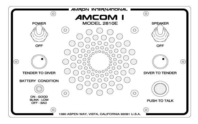
**POWER SWITCH** - The power on/off control.
