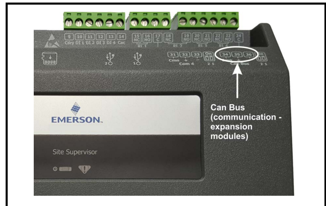
Figure 8-27 - Can Bus Expansion Module
