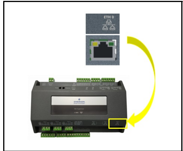
Figure 1-2 - Supervisory Controller ETH0 Port
