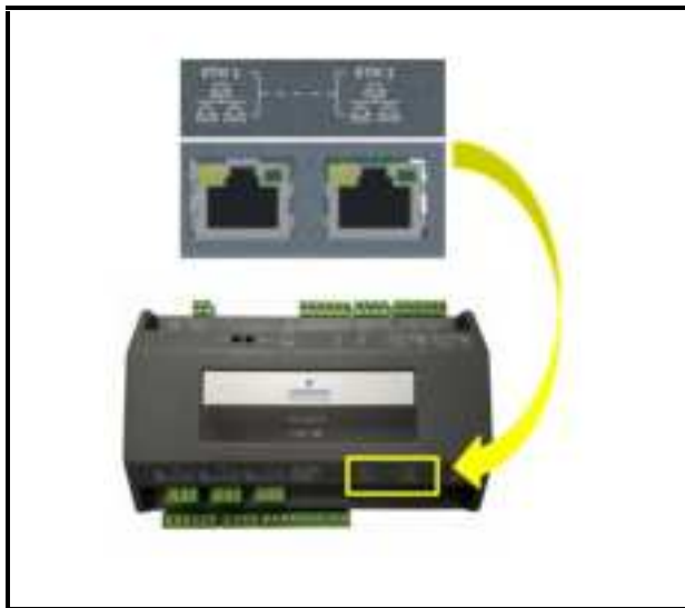
Figure 1-1 - Supervisory Controller ETH1 Ports
