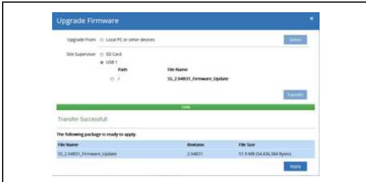
Figure 4-17 - Upgrade Firmware - USB Drive
