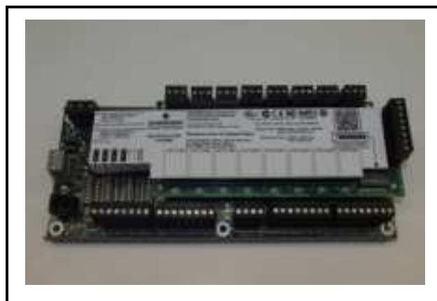
Figure 5-6 - MultiFlex Condensing Unit (CUB)
