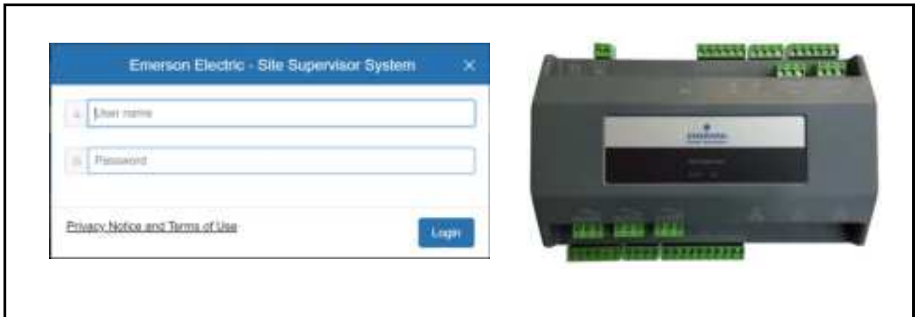
Figure C-1 - Log Into the Supervisory Controller
