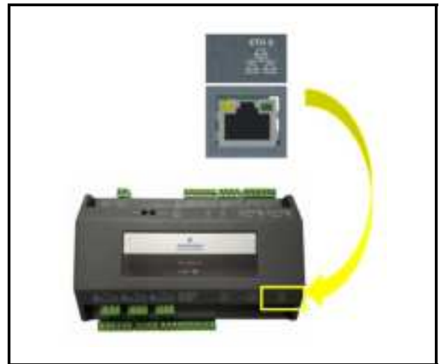
Figure 1-2 - Supervisory Controller ETH0 Port
