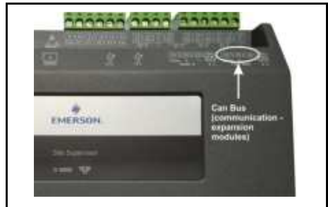
Figure 8-27 - Can Bus Expansion Module
