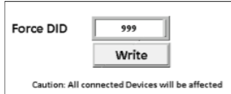
Figure 6. Assigning an ID to an Unknown Device or to All Connected Devices
