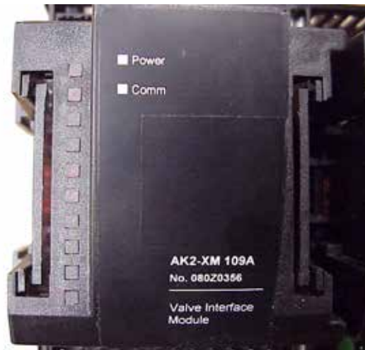
FIG. 33 - POWER AND COMMS LED'S
