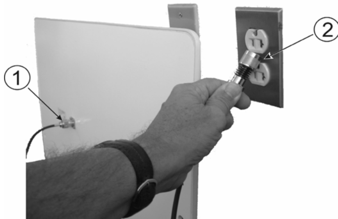
Figure 26 Short Load to Earth Ground
