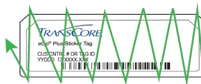
Figure 13 Rub Tag to Bond Adhesive to Windshield
