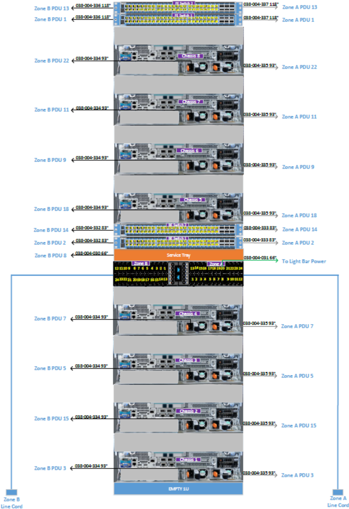
Figure 81 EX3000S three-phase delta AC power cabling
