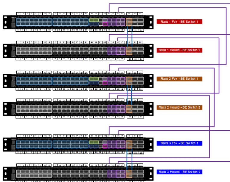
Figure 32 Inter-rack switch connectivity - ring topology
