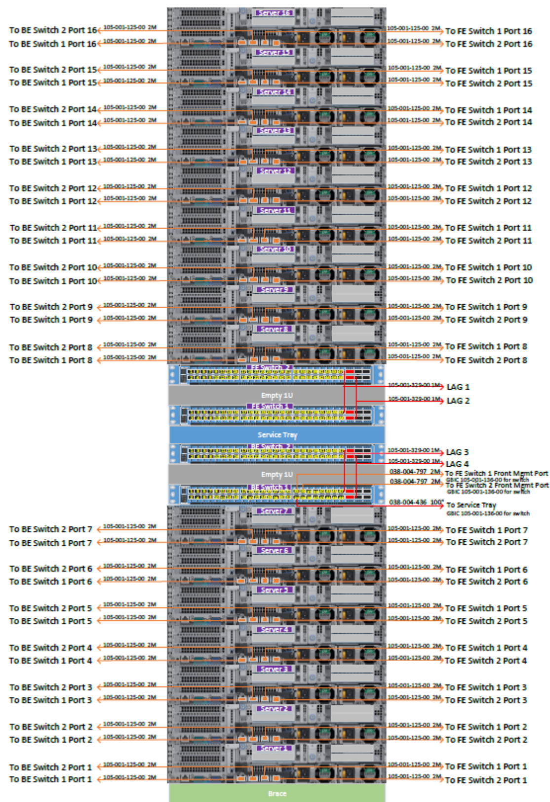
Figure 57 EX300 network cabling
