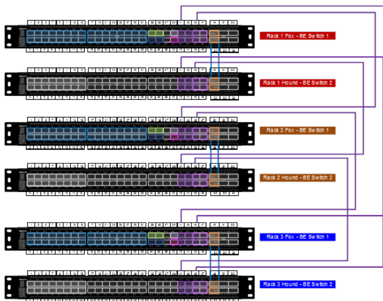
Figure 63 Inter-rack switch connectivity - ring topology
