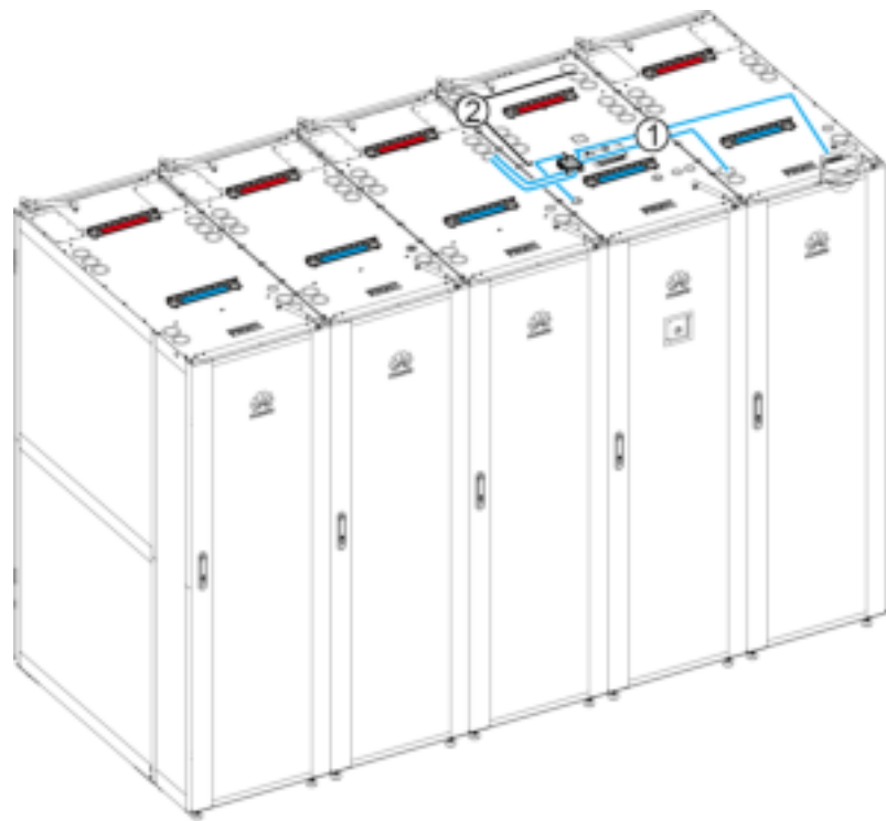
Figure 4-188 Smart ETH gateway cable route
