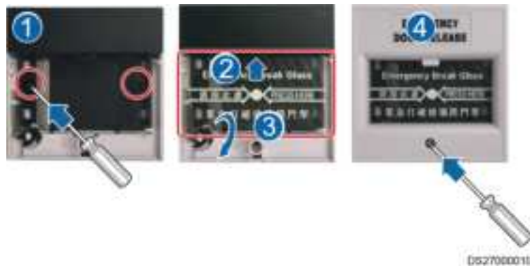
Figure 6-83 Installing an emergency door release button
