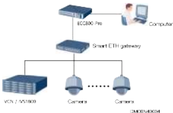
Figure 5-24 Camera + VCN or IVS1800 connecting to the smart ETH gateway
