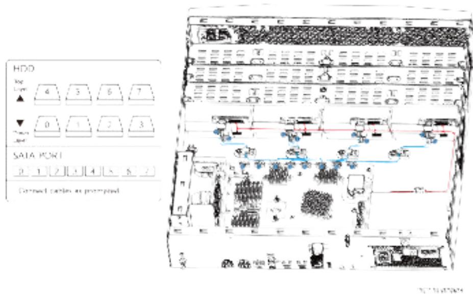
Figure 4-131 Connecting data and power cables to hard disks
