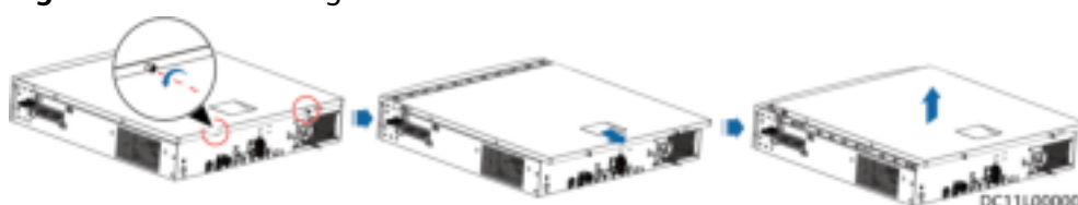
Figure 4-127 Removing the chassis cover
