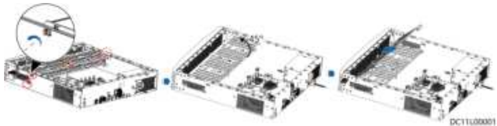
Figure 6-57 Removing the hard disk tray
