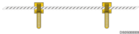
Figure 4-151 Securing a water detection cable
