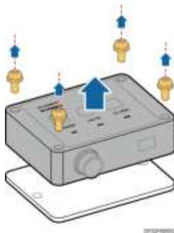
Figure 4-146 Removing the cover from the water detector
