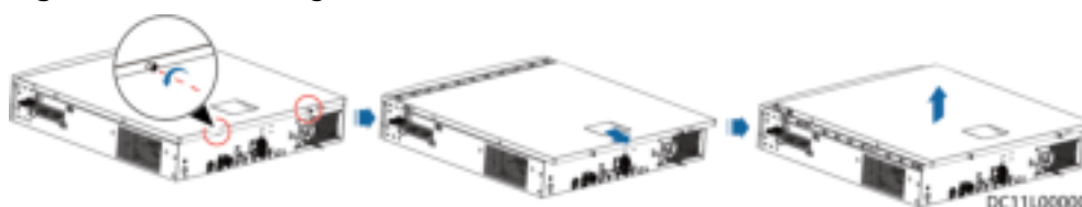
Figure 6-56 Removing the chassis cover
