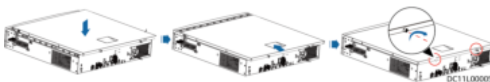
Figure 6-61 Closing the chassis cover
