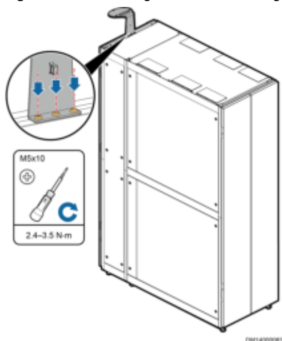
Figure 4-123 Installing a camera mounting plate
