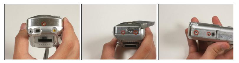
• Locate all five screws on the camera. Then proceed to remove all the screws.
