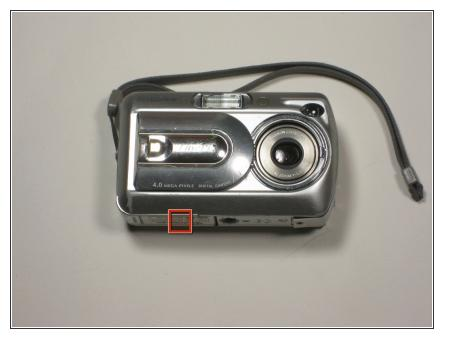
Remove the batteries from the camera to prevent danger of electric shock.
