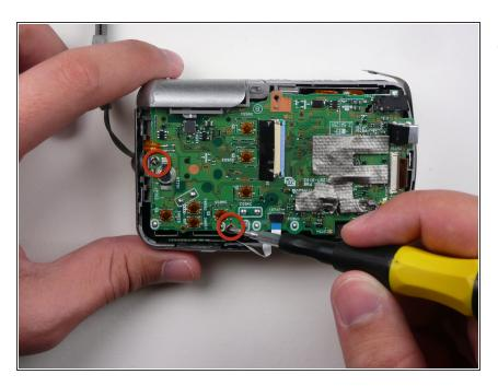
• Remove the two screws holding the circuit board down.
