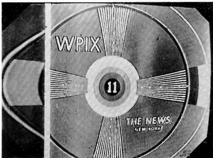
CONDITION—The pattern is non-linear in the horizontal direction with bright vertical bar on left side of screen. CAUSE—Open condenser on one side of the linearity coil.
