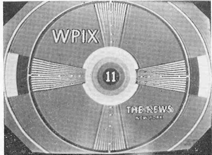
CONDITION:—Poor resolution of the vertical wedges and visible retrace lines (low gain). Trailing white edge in picture. CAUSE:—Use of remote cutoff pentode (6BA6) in i-f strip designed for sharp cutoff pentode (6AG5).
