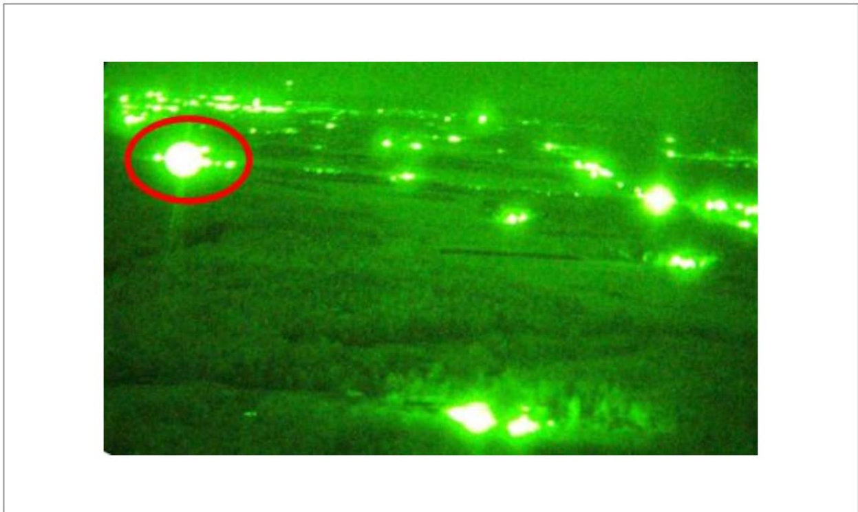
Figure 12-17. Obstruction light (circled) as seen through NVGs (source: National Research Council of Canada)
